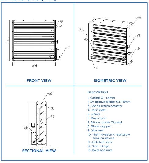
Galvanized steel sheet construction. In accordance with suitable for installation in walls and partitions having leakage class II.
