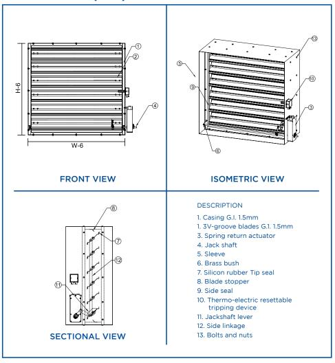
Galvanized steel sheet construction. In accordance with UL555S suitable for installation in walls and partitions having leakage class II.
